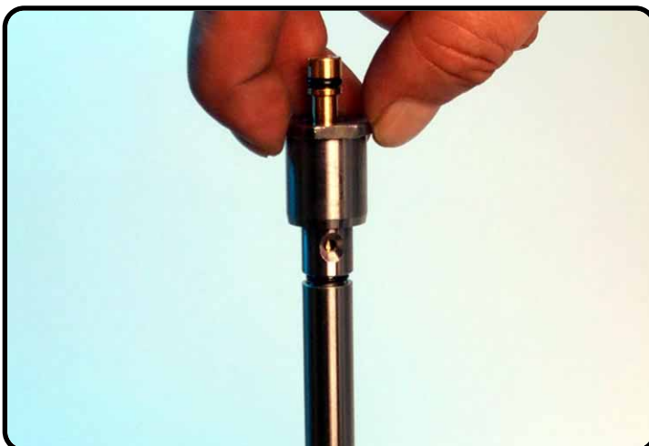
Clamp the piston rod in on the other side and screw in the piston rod adaptor.
