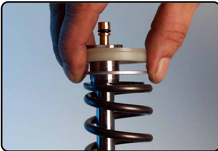
Replace the steel washer first and then the preload spacers.
