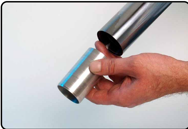
Hold forkleg up side down and remove the house hydraulic stop.
