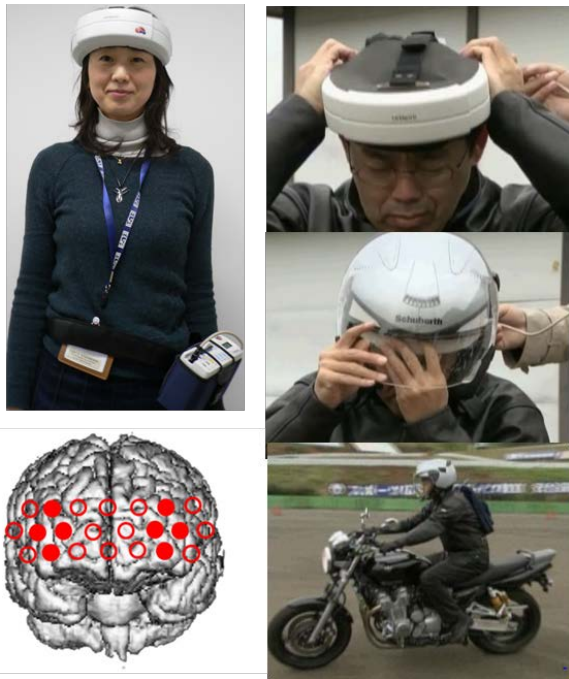
Fig. 1 A prototype of the wearable optical topography (WOT) system and the location of the system's measurement points. A probe unit of the WOT system can be accommodated on the head of the subject, and a processing unit can be strapped to the subject's body. During the experiments, the subjects were asked to wear a helmet over the probe unit of the WOT system. 22 measurement points (red circles) cover the area around the dorsolateral prefrontal cortex. We selected four channels covering the DLPFC in each hemisphere (red filled circles) for statistical analyses.
